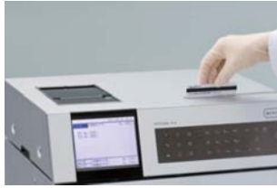
Calibration by magnetic card
